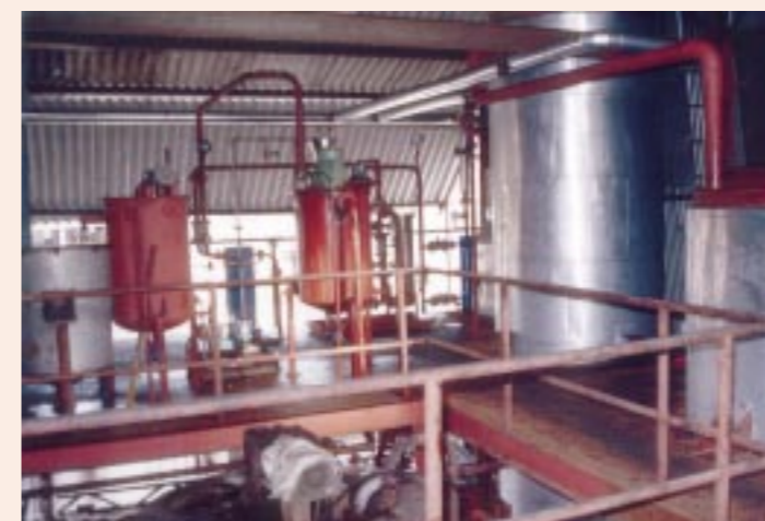
Enzymatic degumming section in a rice bran oil refinery
