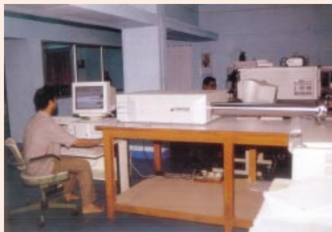
Matrix Assisted Laser Desorption Ionization Time of Flight (MALDI TOF) Mass Spectrometer (Model: TO-4X KOMPACT SEQ, KRATOS, UK)
