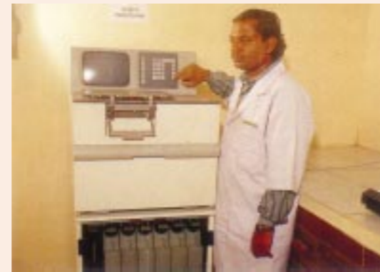
Tissue Processor (Model: HMP 300, Microm GmbH, Germany)
